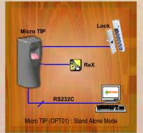
Model: MicroTIP(OPT 01): Stand-alone Access Control System in Identification Mode (1:N) Mode
